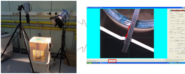
Fig. 4 Maximum displacement measurement using a super-high speed camera
