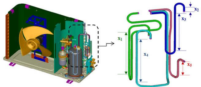
Fig. 5 Analysis model and five design variables of air-conditioner pipe design problem
