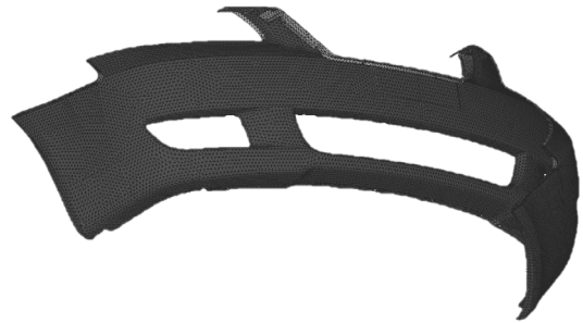
Fig. 1 Finite element model of the front bumper
