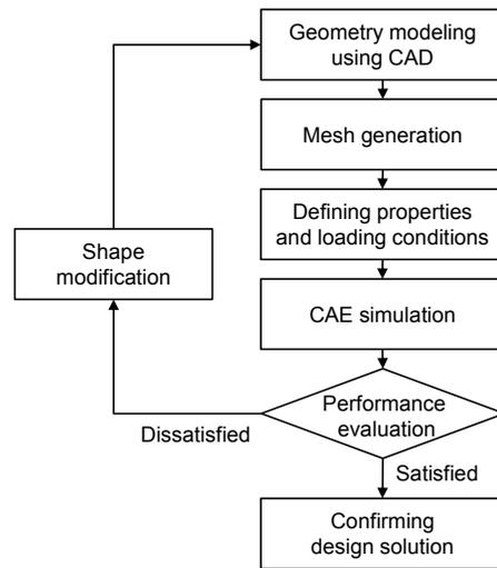
Fig. 6. Traditional procedure of shape design.
