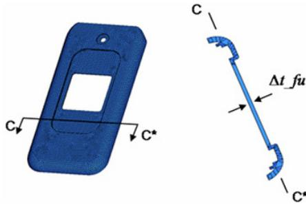
Fig. 4. Shape variable for thickness of folder upper.
