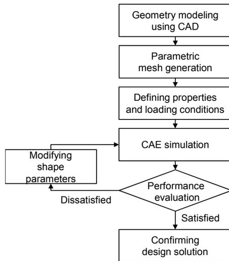
Fig. 7. Procedure of shape design using mesh morphing.
