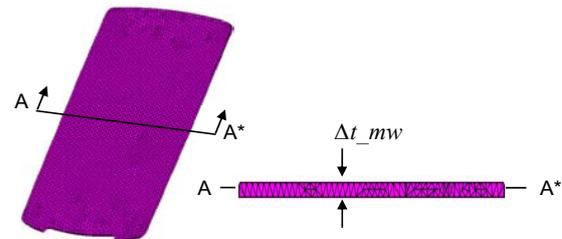
Fig. 2. Shape variable for thickness of main window.
