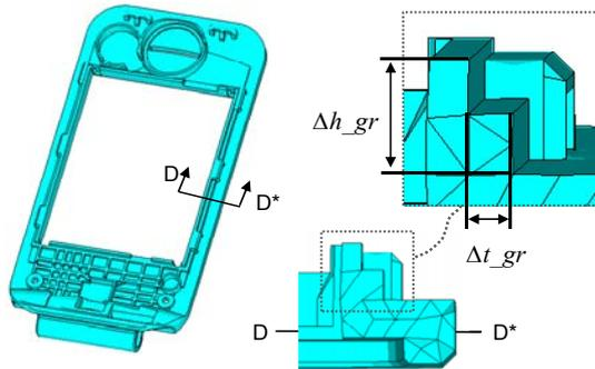
Fig. 5. Shape variable for thickness and height of guide rib.
