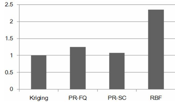
Fig. 10. Normalized cross-validation errors for metamodels.
