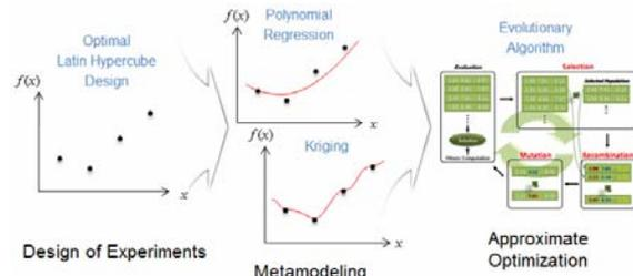
Fig. 11. Metamodel-based optimization procedure.
