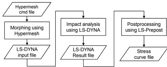
Fig. 9. Analysis processes of impact simulation.
